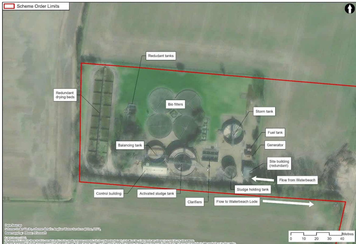
Figure 8.3: Schematic of the Waterbeach WRC
